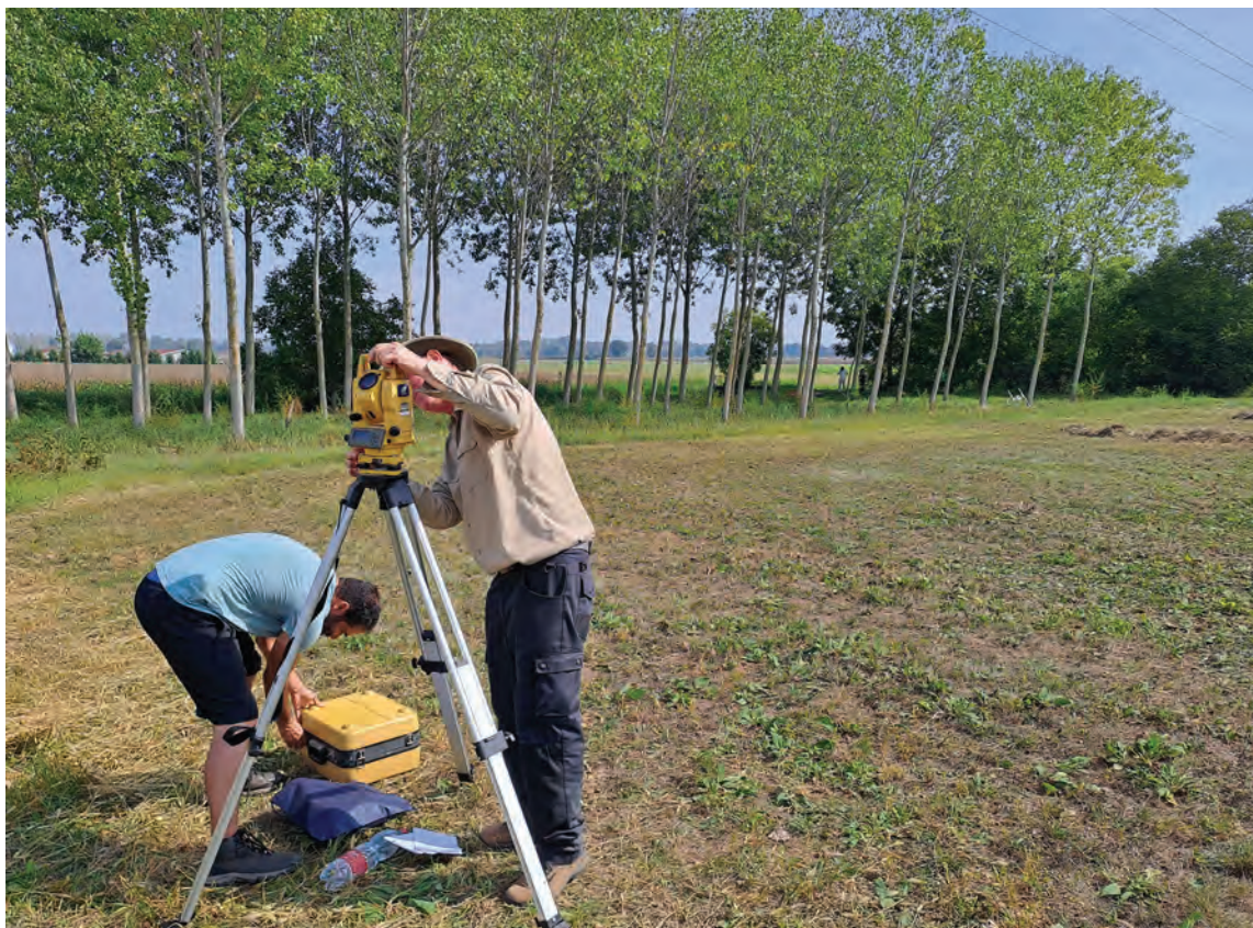
Figure 5. Hans Barnard (right) sets up a total station with the help of UCLA graduate student Brandon Keith.
