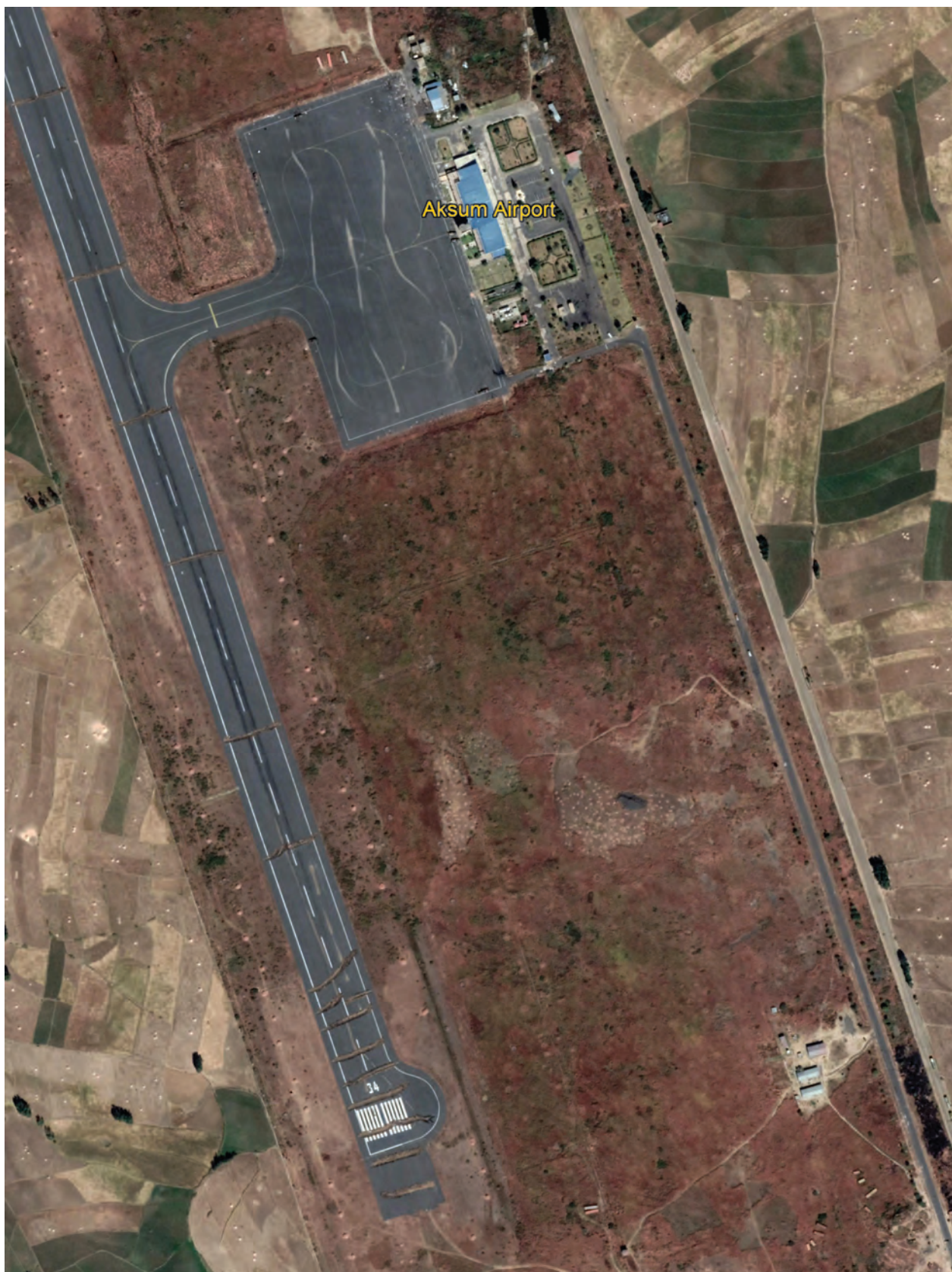
Figure 5. Satellite image of Aksum Airport, Tigray, November 2020. Note the walls built across the runway to render it inoperable. (Image courtesy of Maxar Technologies/Google Earth.)
